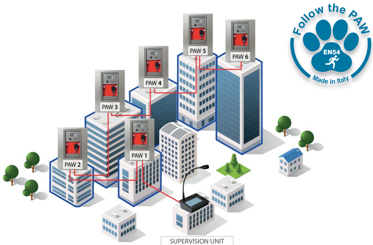
This application example demonstrates the use of 6 intercommunicating PAW systems in the installation of a complex made up of several buildings.
